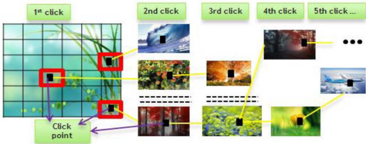
Fig 2. In CCP, user selects one click-point per image. The next image displayed is determined by the current clickpoint.
